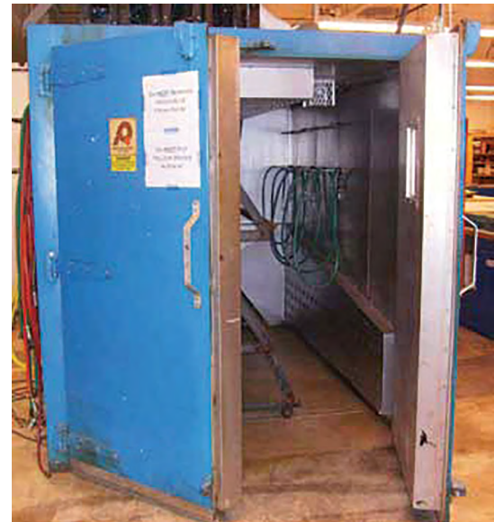
Figure 3-32. Walk-in curing oven.
