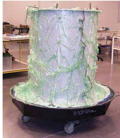
Figure 3-31. Bagging of complex part.
