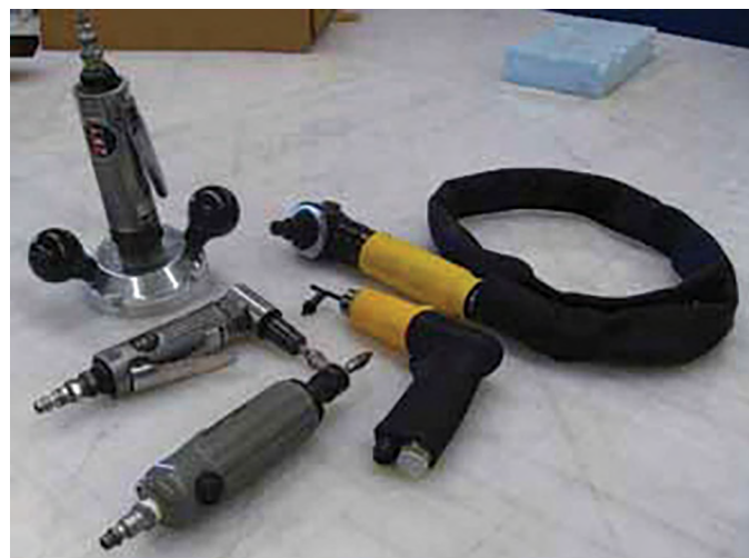
Figure 3-27. Air tools used for composite repair.
