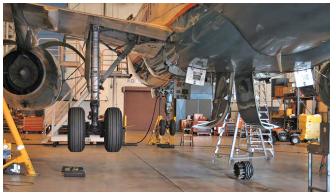
Figure 2-28. Airbus A-320 being jacked.
