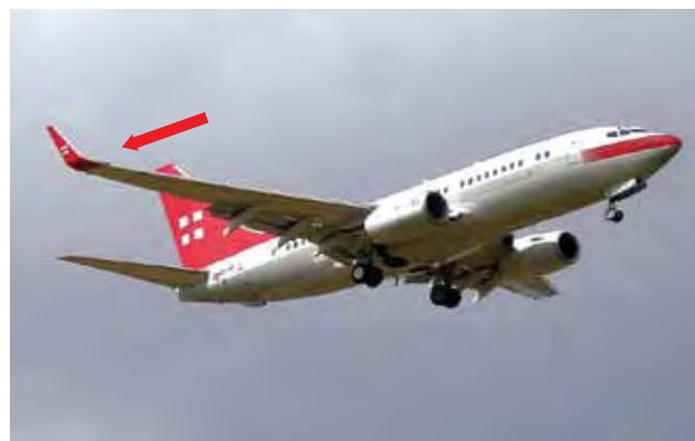
Figure 1-40. A winglet reduces aerodynamic drag caused by air spilling off of the wing tip.
