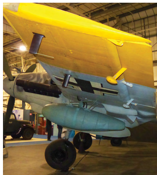
Figure 1-32. An aileron mass balance.
