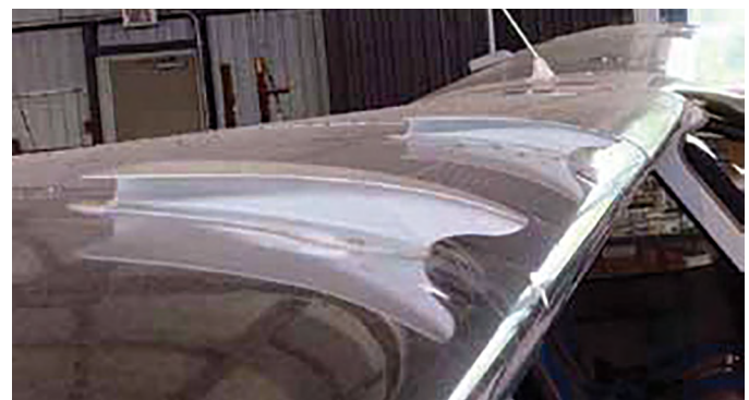
Figure 1-37. The Symphony SA-160 has two unique vortex generators on its wing to ensure aileron effectiveness through the stall.
