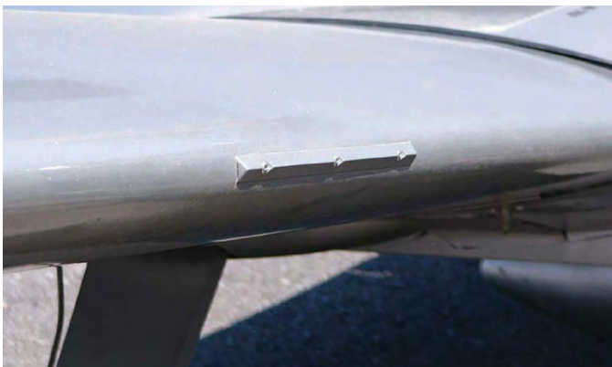
Figure 1-38. A stall wedge causes the wing root to stall before the outboard wing. This preserves airflow over the ailerons for controlled recovery from the stall.
