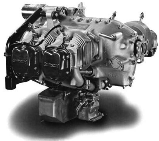
FIGURE 1-11 Continental Motors 200 series engine.
