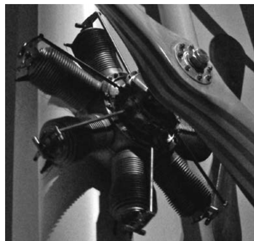
FIGURE 1-2 Gnome-Monosoupape rotary engine.
